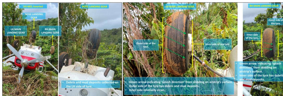
Figure 9: Debris and mud deposits on the tyre indicating how the aircraft drifted during ground loop.
