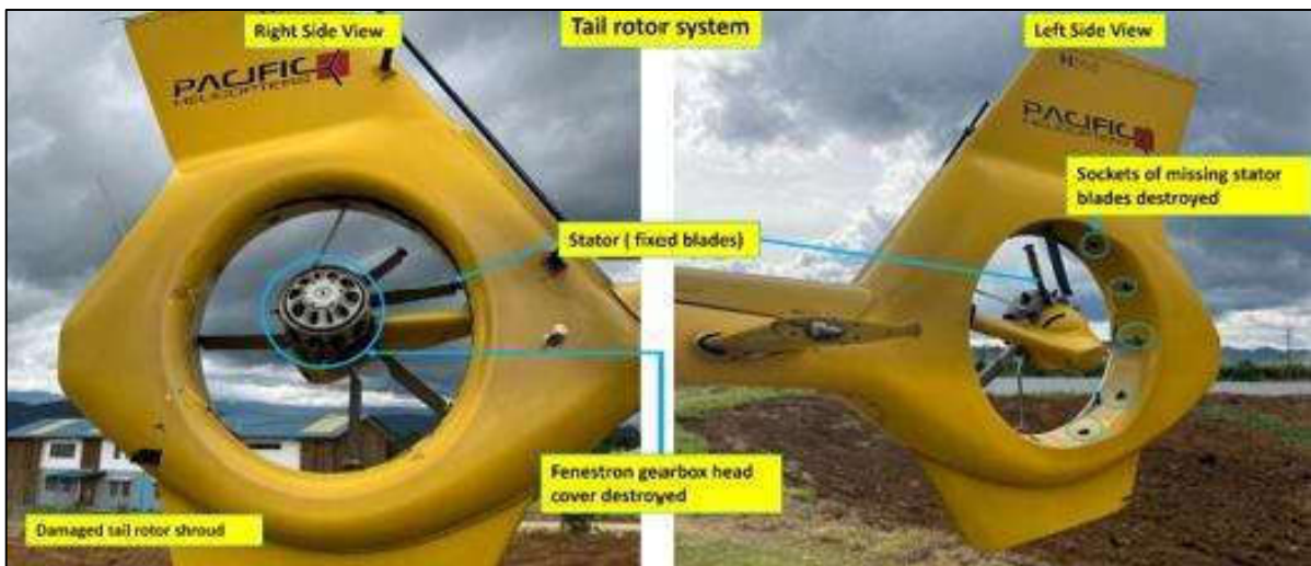
Figure 7: Damage sustained to the fenestron and its components
