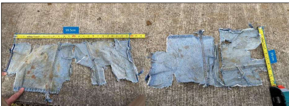
Figure 8: FOD - Pieces of the denim material
