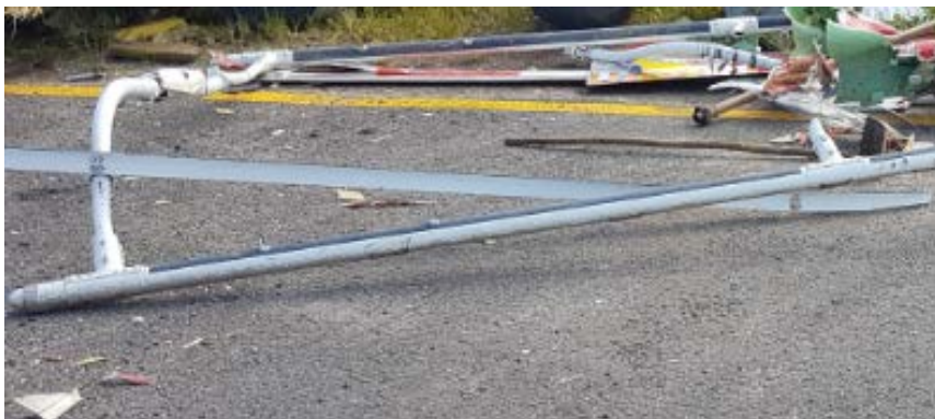
Figure 4: Separated landing gear skid assembly
