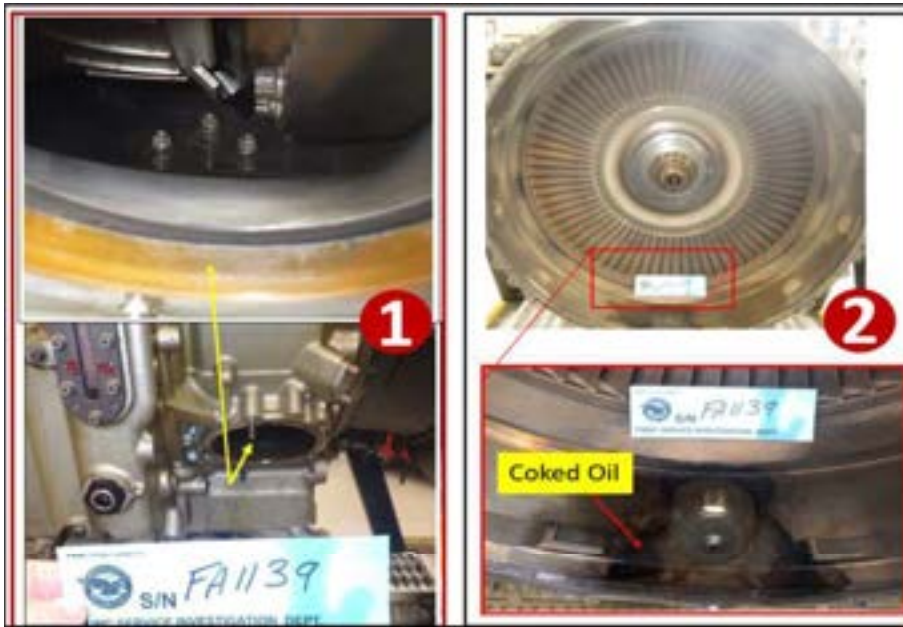
Figure 5. LP compressor(1) and turbine support case(2)
