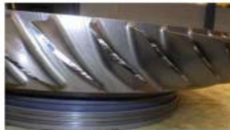
Photo No. 47 3 rd stage LPC rotor
