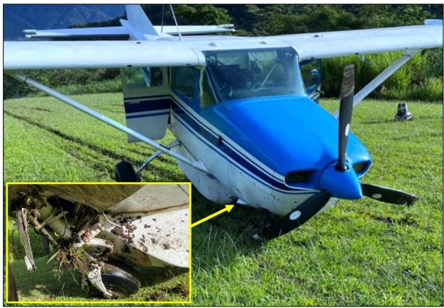
Figure 4: Overview of the damage sustained during impact
