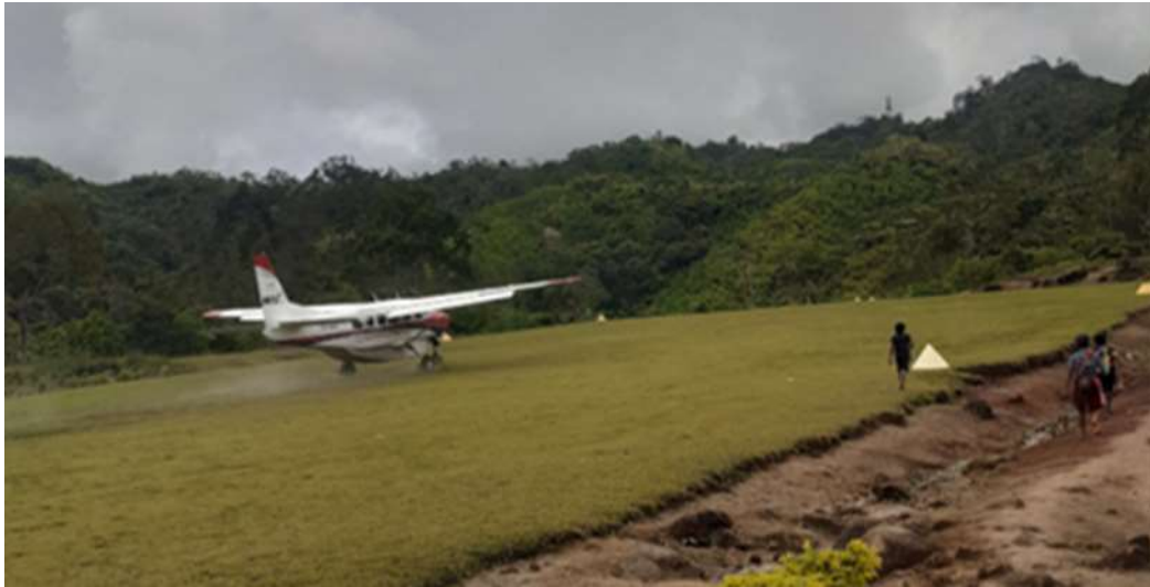
Figure 3: Water on airstrip coming out from under the tyres of P2-MAF during landing roll. (Source: Witness)
