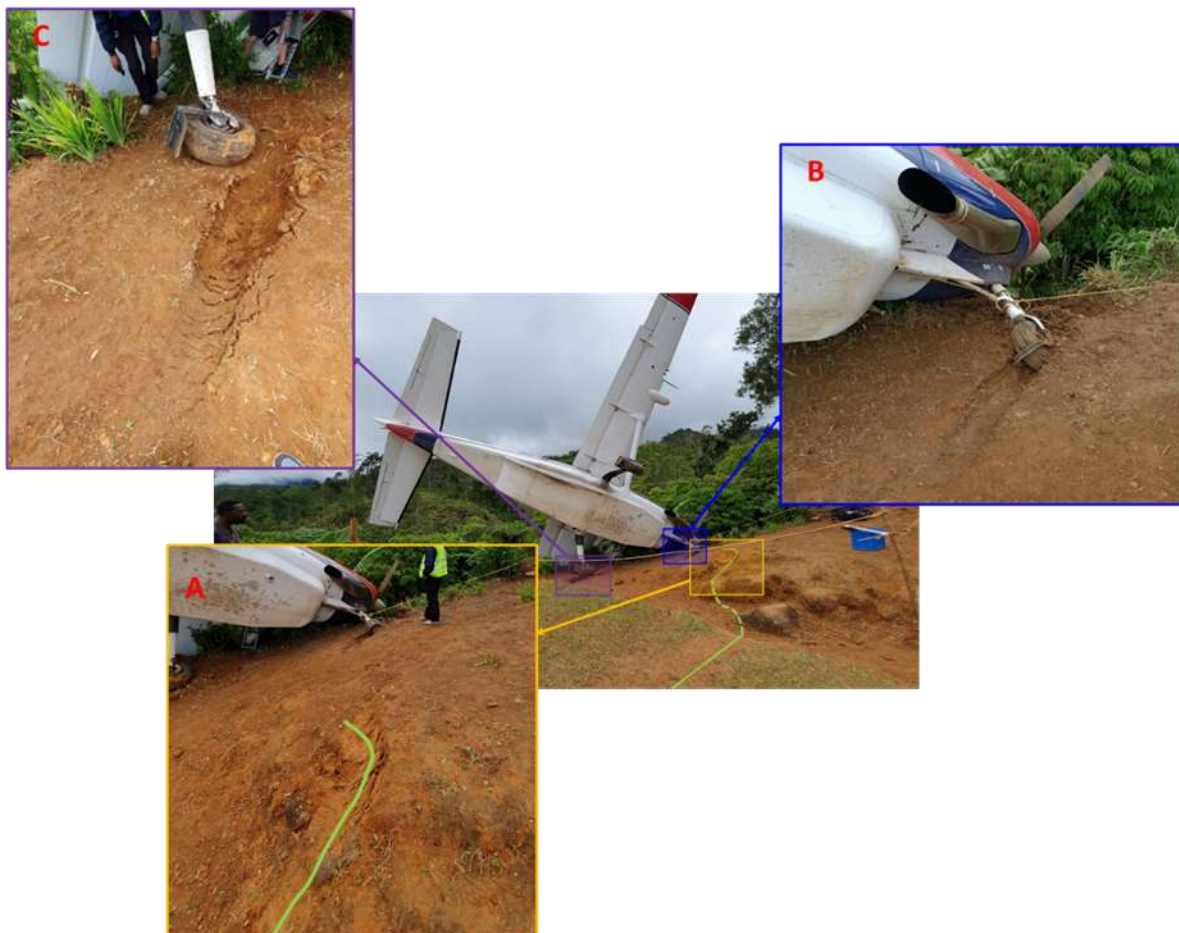
Figure 12: A- Overrun impression of right main wheel on end of airstrip; B- Nose wheel dug; C- Left main wheel.
