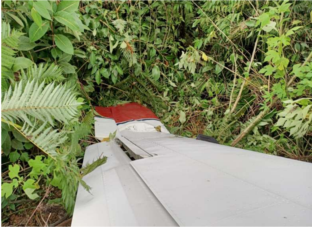
Figure 6: Left wing impacted ground in gully.
