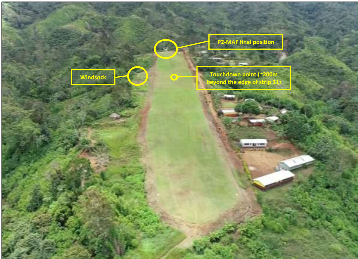
Figure 2: Overrun illustration of P2-MAF at Yenkisa Airstrip.
