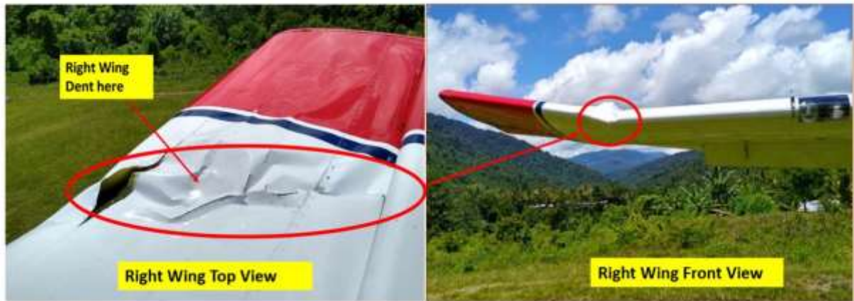
Figure 4: Damage to right wing
