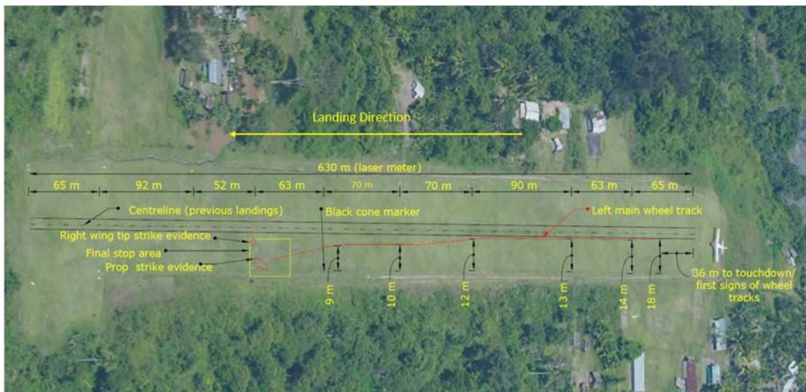
Figure 6: Overview of landing roll track-Full length (Source MAF PNG)
