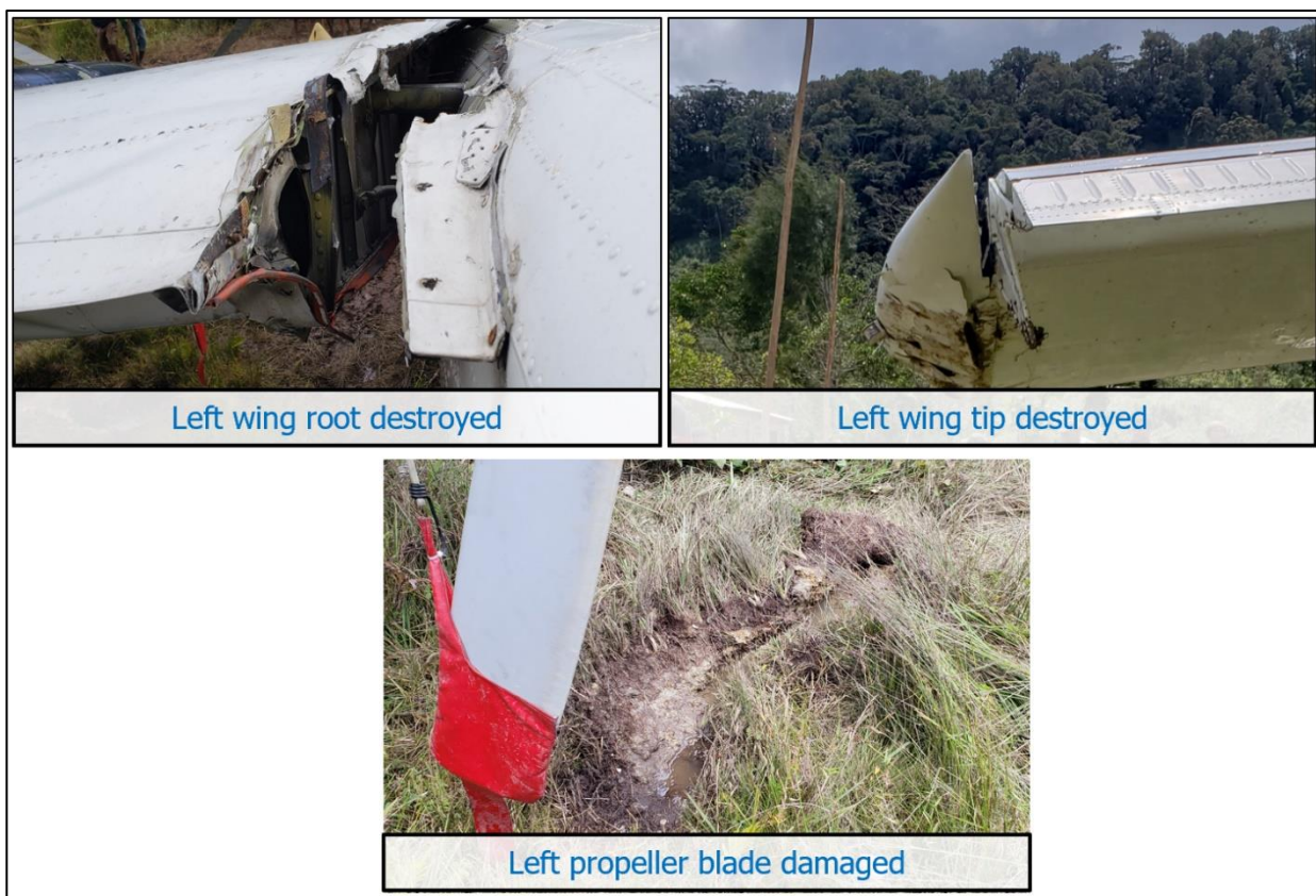
Figure 4: Damage sustained at the left-hand side of the aircraft
