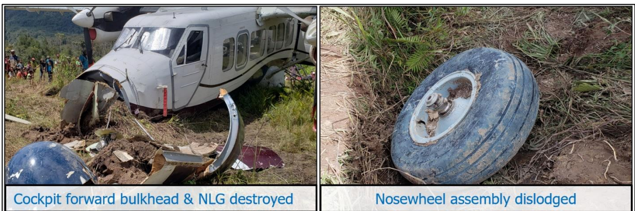
Figure 3: Damage sustained at the Nose section
