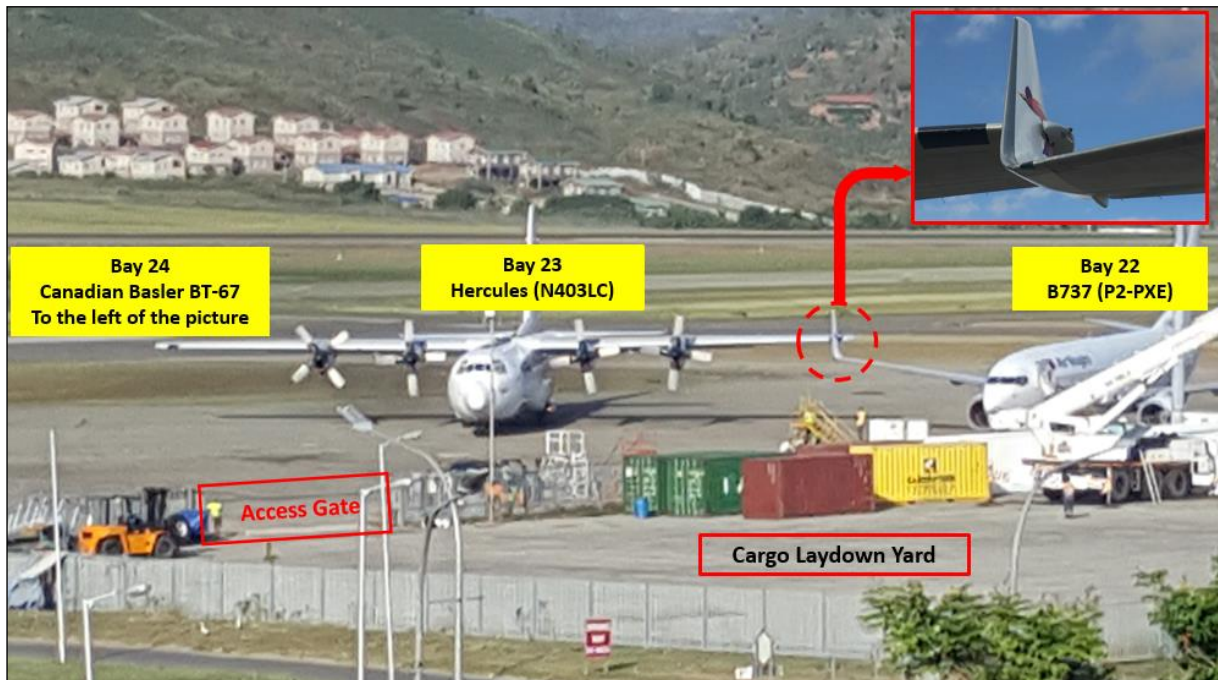
Figure 2: Wings collision damage (Source: Eye witness)
