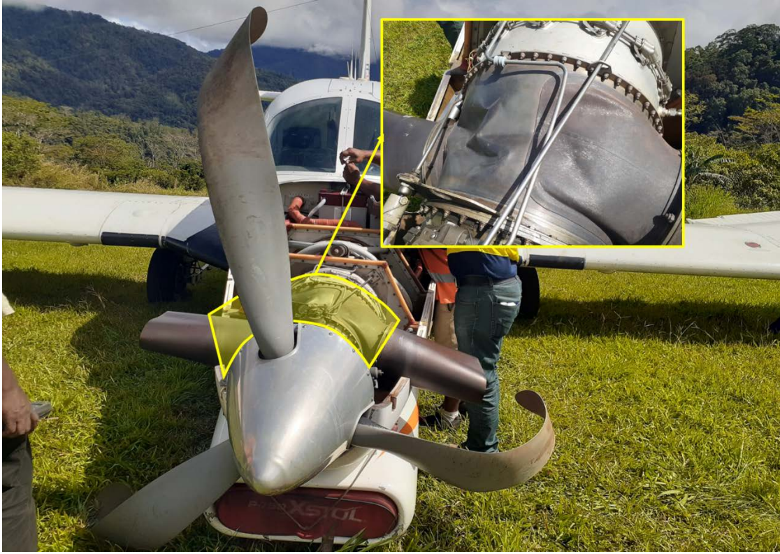
Image 4: Insert shows engine reduction gearbox and exhaust zone.
