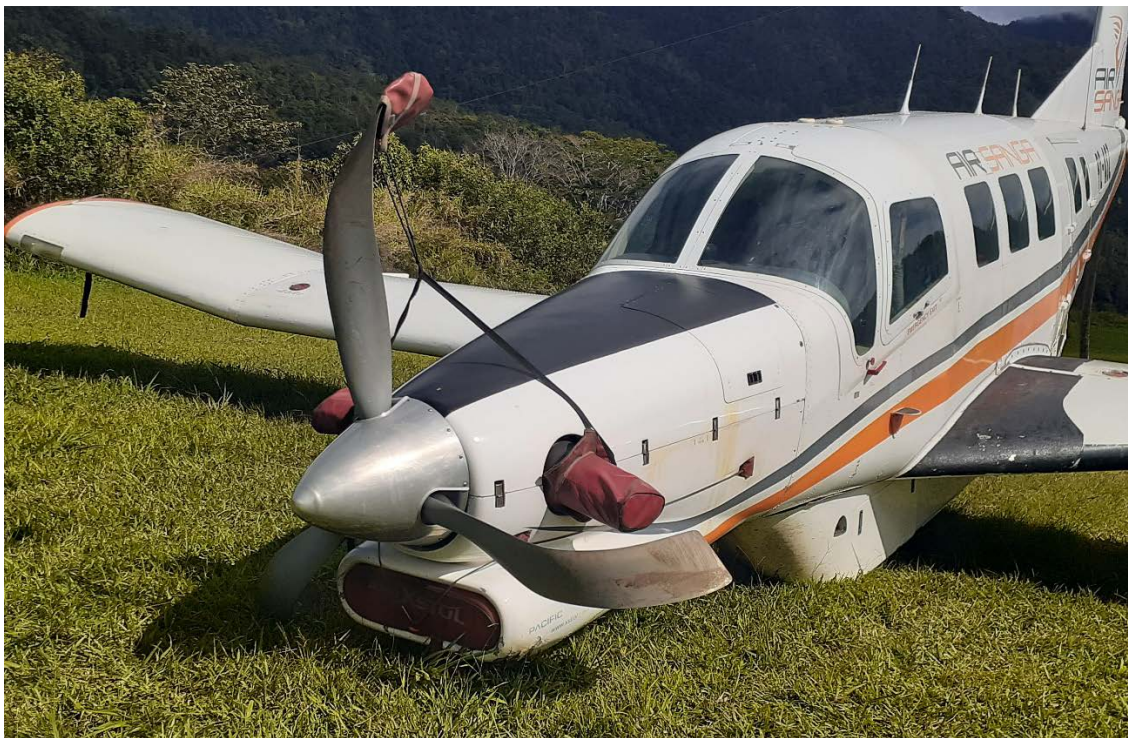
Figure 3: View of the damaged propeller and nosewheel zone.
