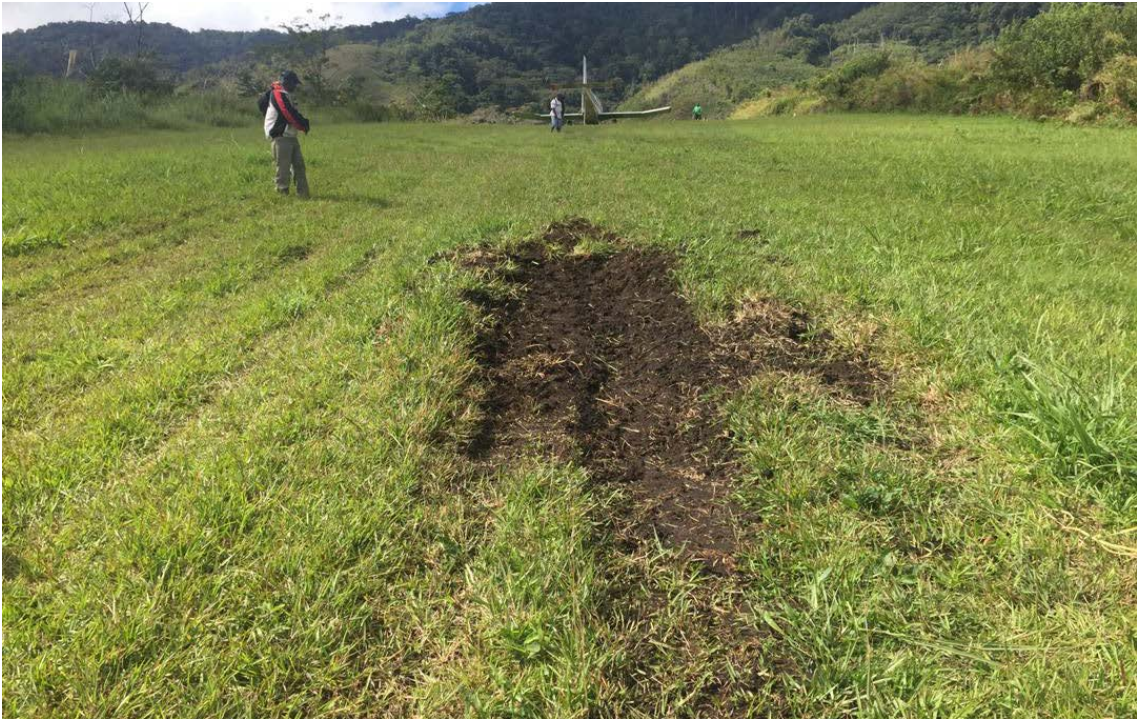
Figure 2: Impact nosewheel mark and the aircraft in its final position.
