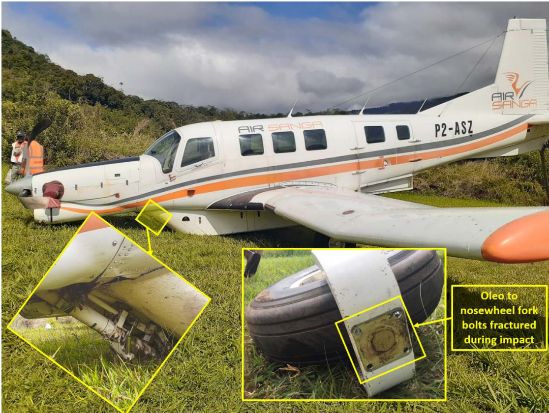
Image 5: Nose landing gear assembly folded back into the cargo pod
