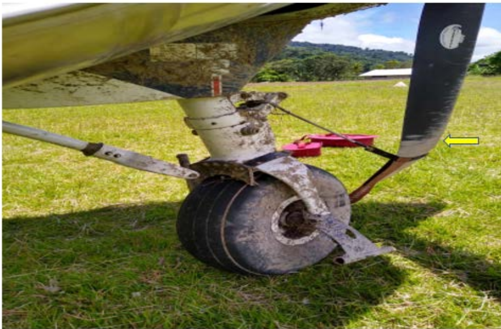
Figure 5: Evidence of damage in a propeller blade
