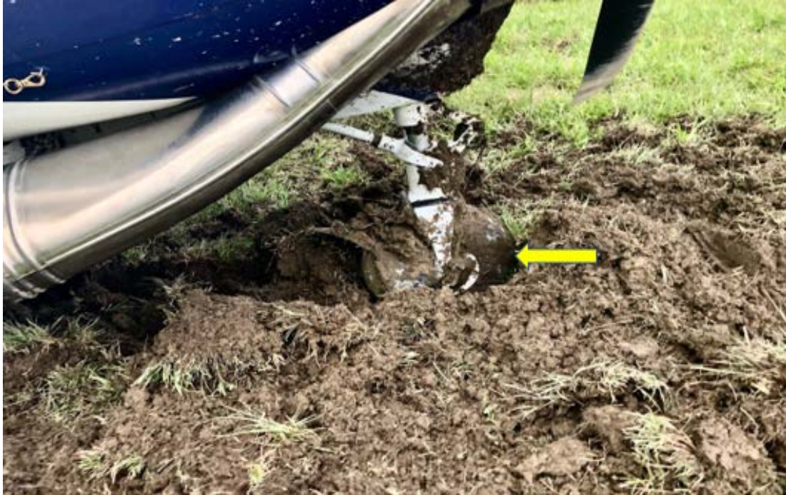
Figure 2: Nose wheel bogged in soft mud
