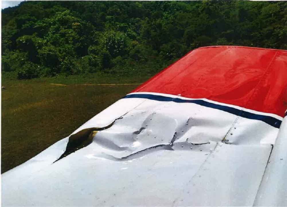
Figure 4: Right-hand wing tip damage
