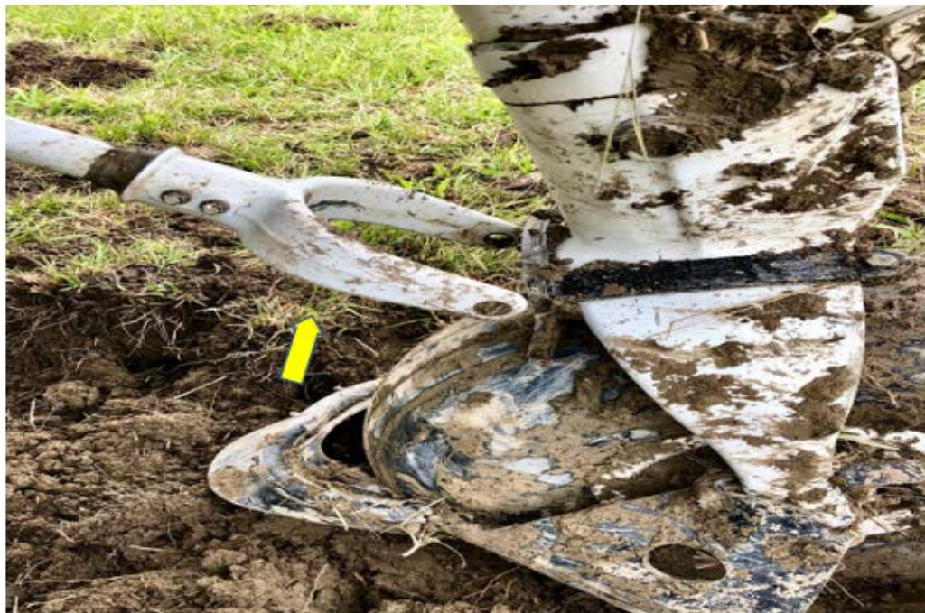
Figure 3: Detached NLG Spring from nose wheel landing gear
