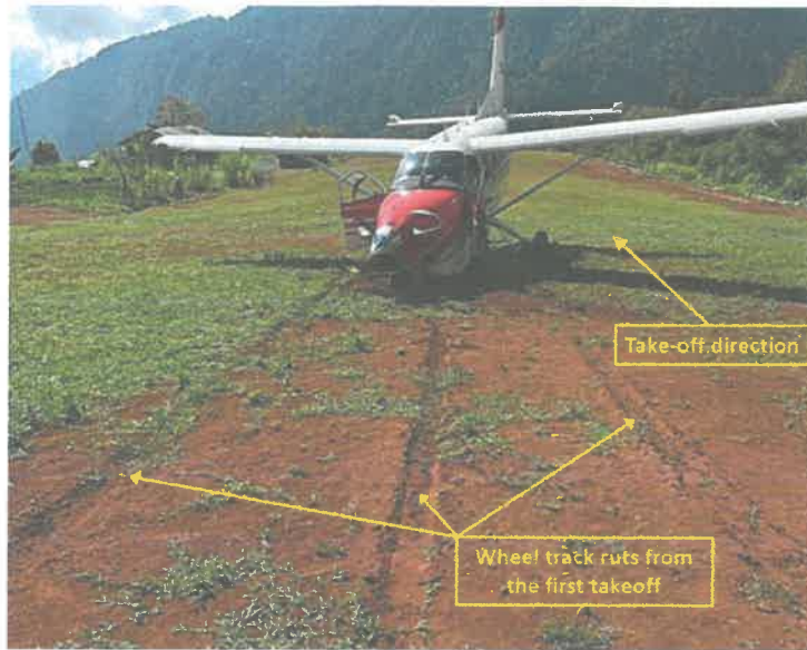
Figure 2: View of P2-NTZ showing the ruts in the soft strip surface from the first takeoff
