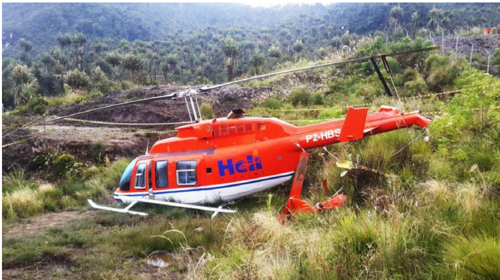
Figure 3: Bent skids and severed tail boom as a result of heavy landing
