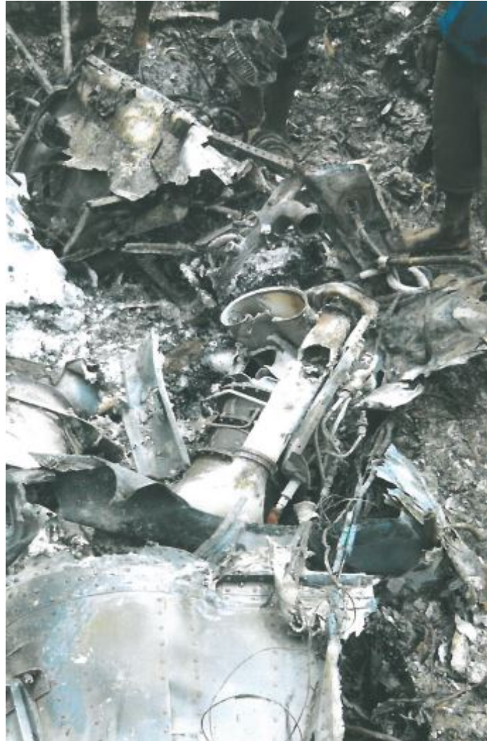
Figure 2: Cockpit and engine destroyed by the fire
