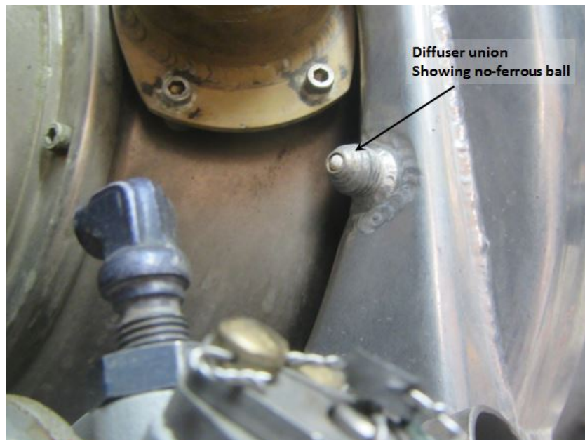
Figure 7: The ‘foreign object’ stuck on inside of the union mount on diffuser
