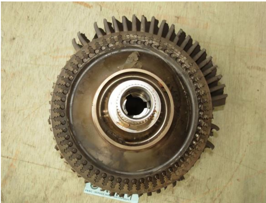
Figure 8: CT disk and blades upstream side
