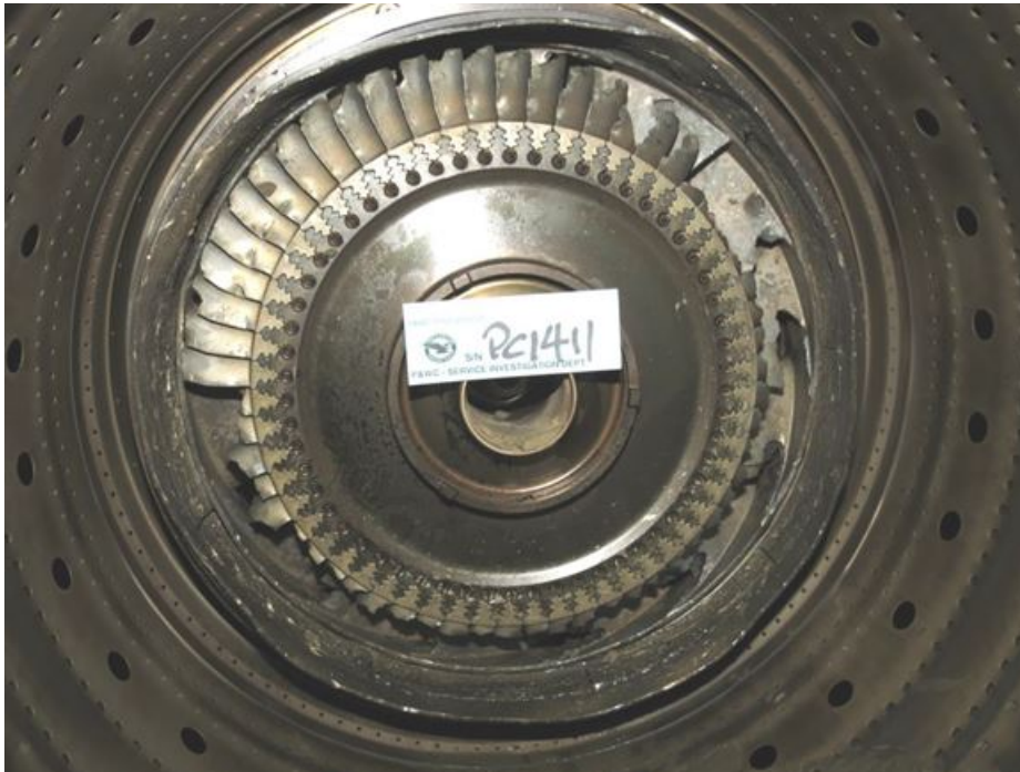
Figure 8: CT disk and blades downstream side
