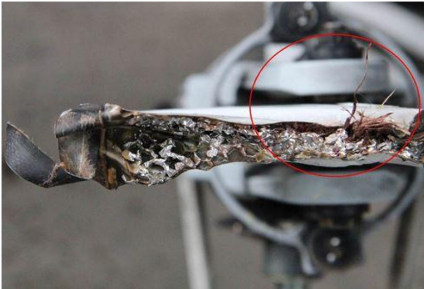
Figure 17: Tail rotor blade root with wood fibres in the fracture surface
