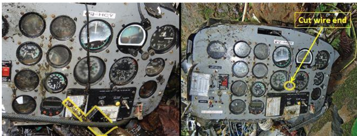
Figure 10: HCY instrument panel at the accident site Source: Australian Army
