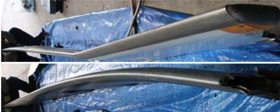
Figure 13: Main rotor blade deformation upward and downward respectively
