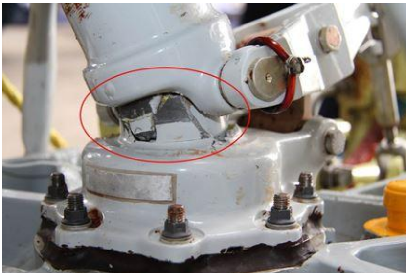
Figure 16: Fractured swashplate support
