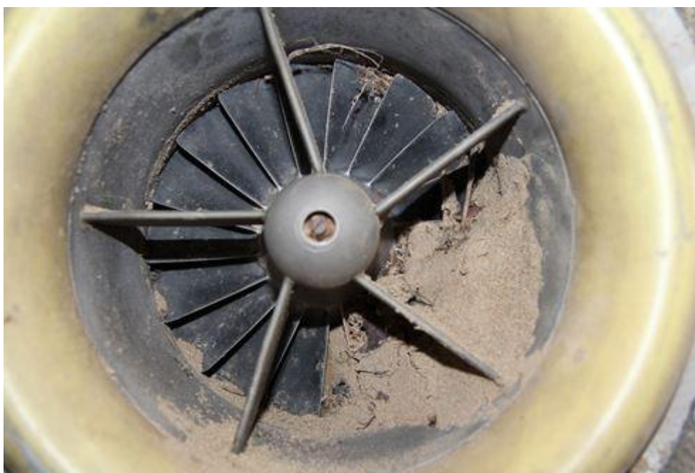
Figure 25: Sand/silt in the compressor inlet
