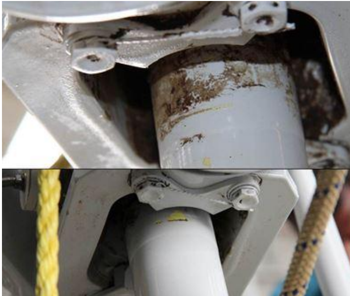
Figure 15: Static stop contact area on either side of the main rotor mast
