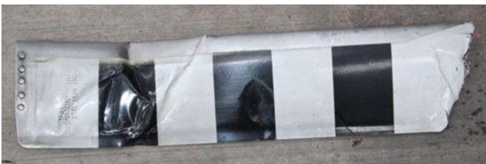
Figure 18: Tail rotor blade displaying a compression load from tip to root
