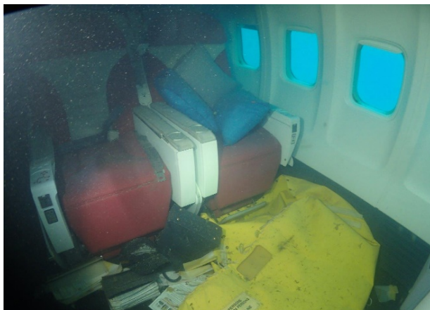
Figure 22: 56-person life raft cover on the floor in front of Business Class Seats 1A and 1B. (Photo taken by FSM diver)
