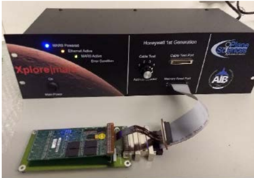
Figure 49: SSFDR memory chip board connected to Memory Access Retrieval System (MARS)
