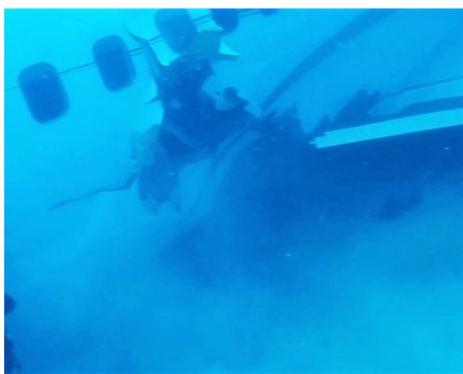
Figure 16: Fuselage fracture right side behind the wing showing wing flap separation
