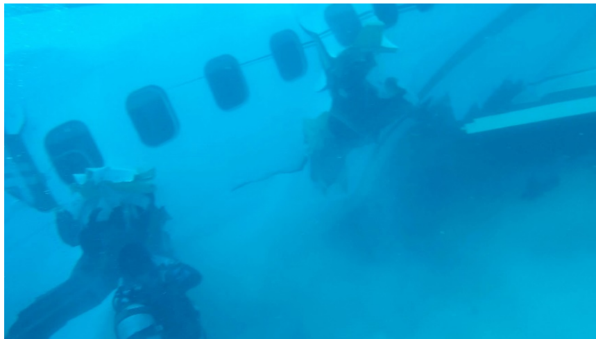
Figure 15: Fuselage fracture right side behind the wing at wing root, in the area of seat row 22
