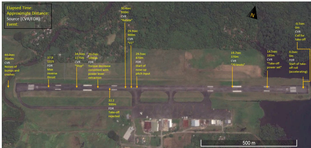
Figure 12: Madang runway with position of FDR and CVR recorded events (See Appendix 1 for enlarged diagram for clarity)
