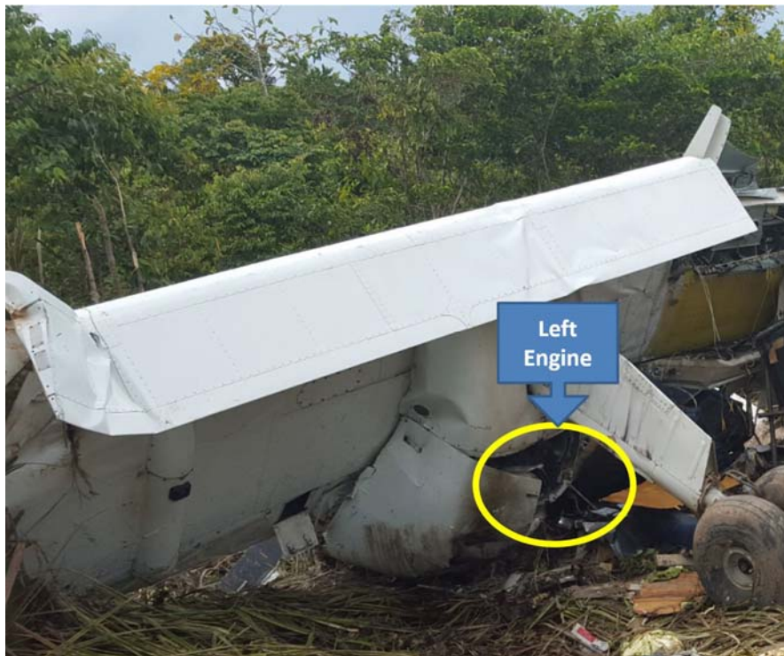
Figure 15: Left engine still attached to its mount
