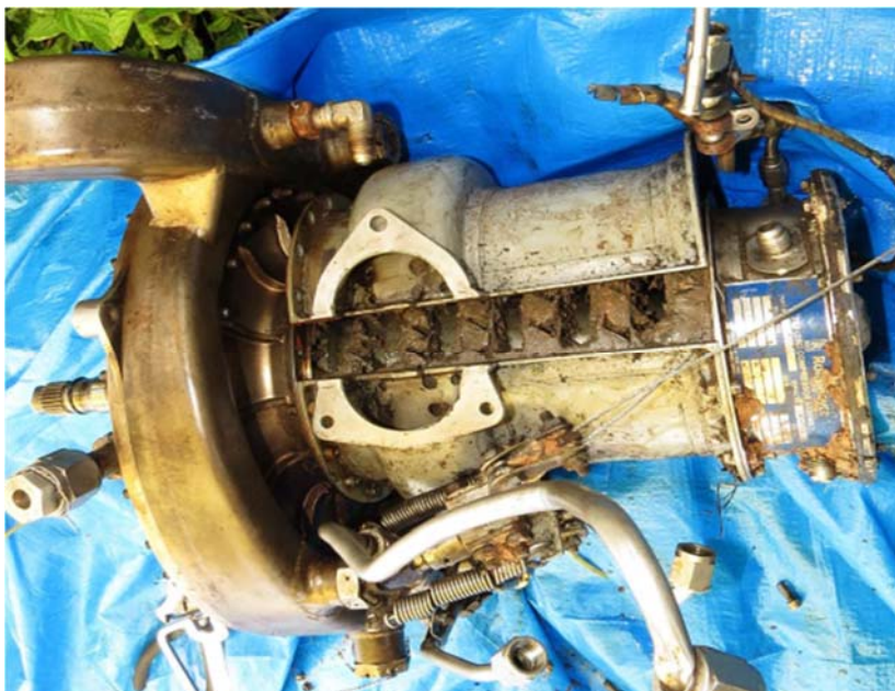
Figure 29: Compressor module, removed from right engine
