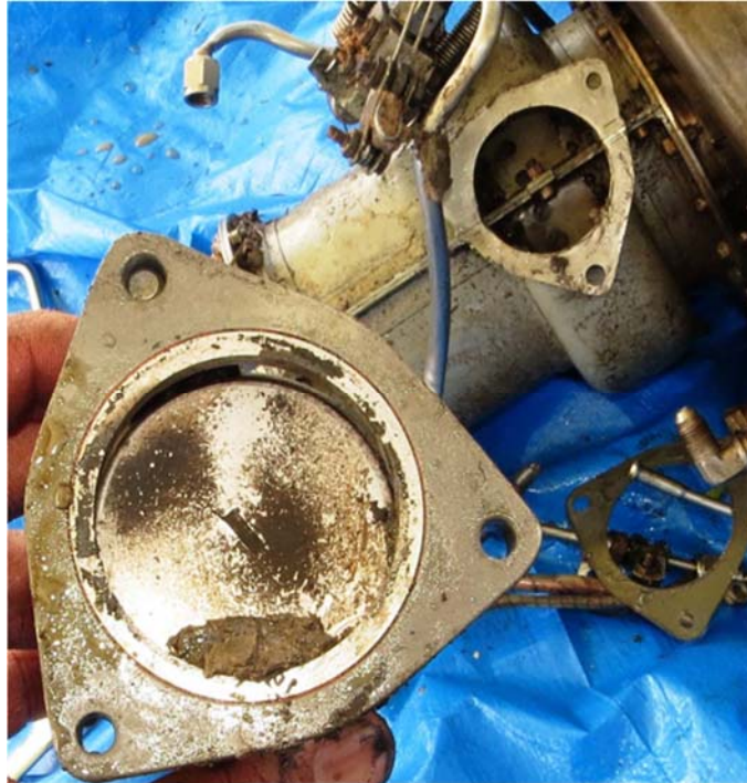
Figure 32: Bleed valve face (Source: Rolls-Royce Corporation)
