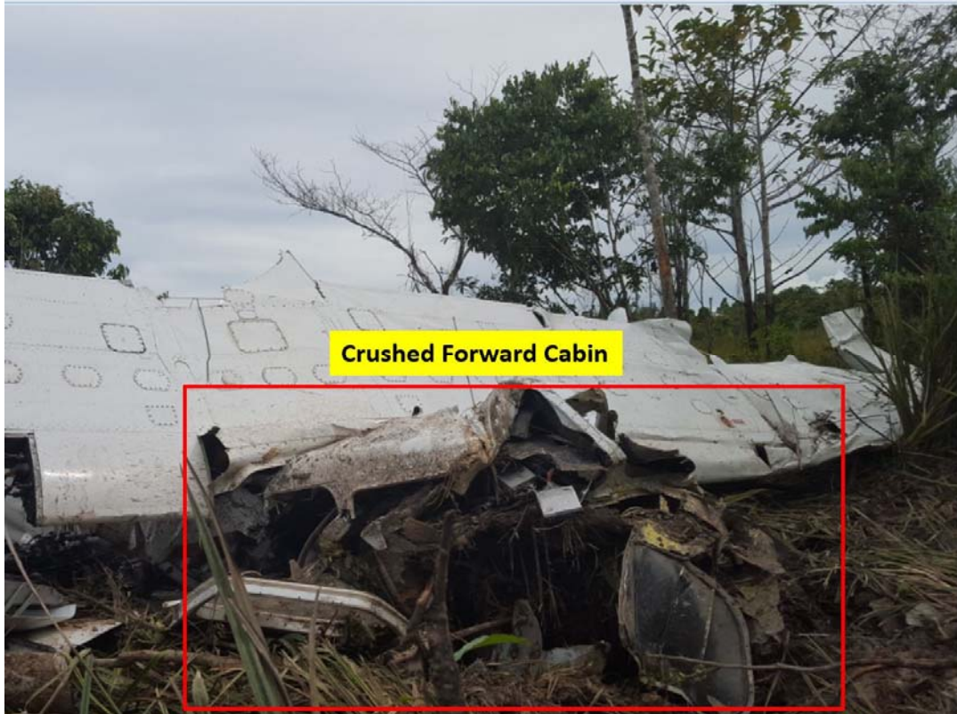
Figure 12: Compressed Forward Cabin
