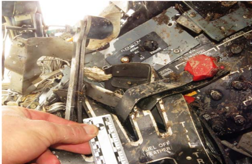
Figure 21: Power and Control Lever approximately 4cm above IDLE
