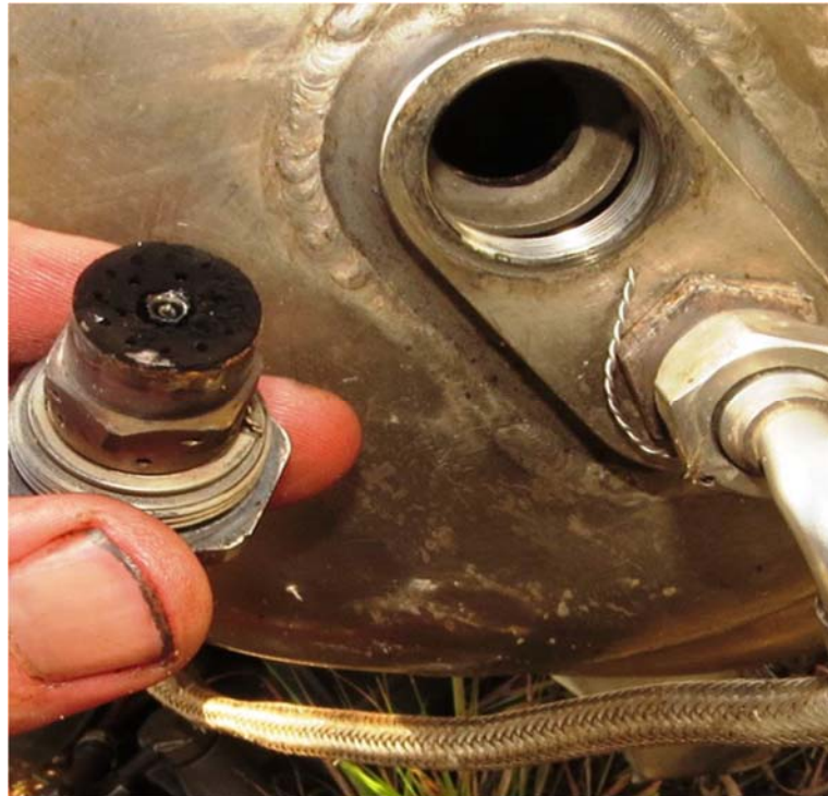
Figure 26: Left engine fuel spray nozzle removed from combustor
