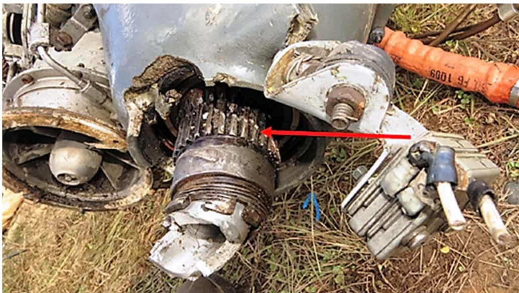
Figure 24: Spiral disengagement witness marks (arrows) on the left propeller drive shaft
