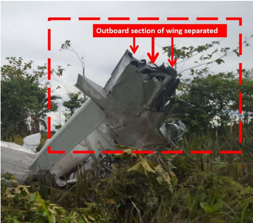
Figure 18: Right wing outboard of the engine nacelle separated
