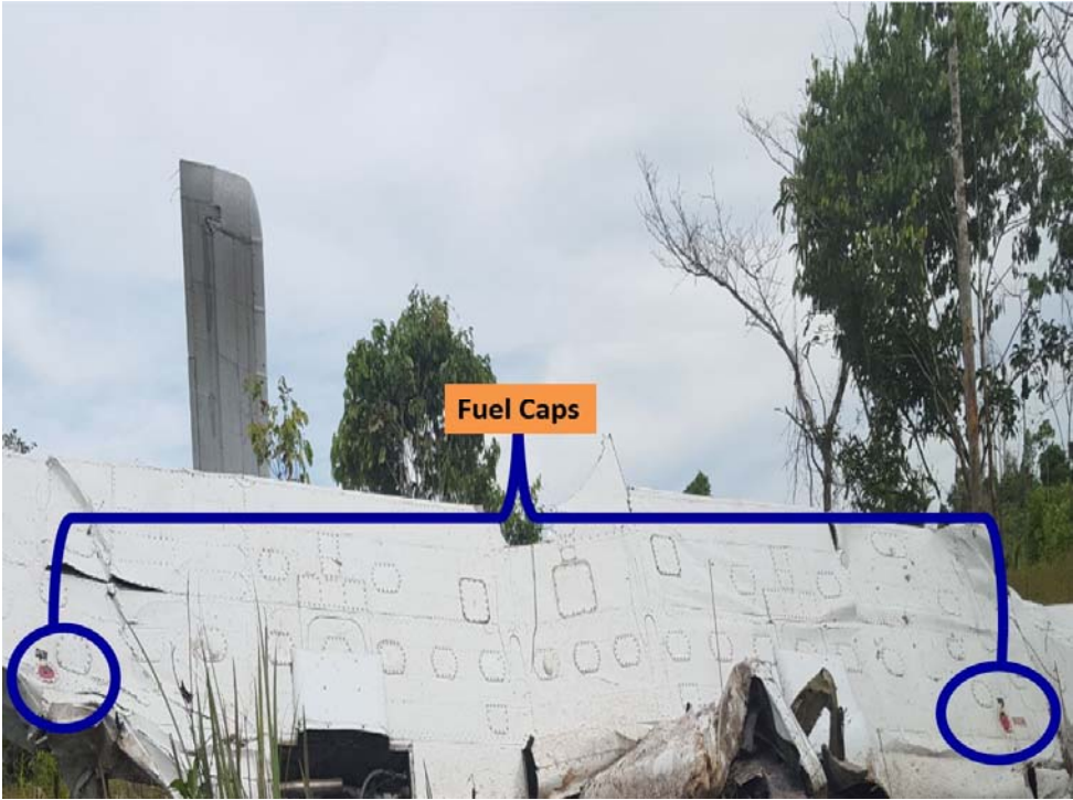
Figure 19: Wing assembly showing caps of both fuel tanks secured
