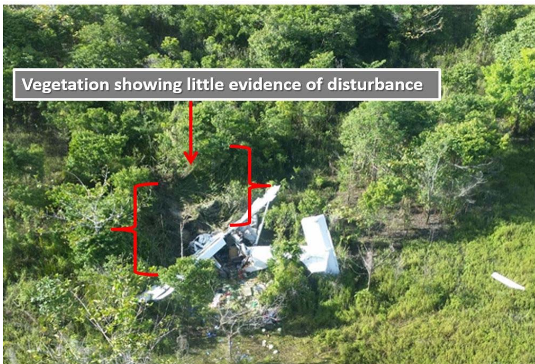
Figure 9: Accident site showing wreckage confined to general dimensions of the aircraft
