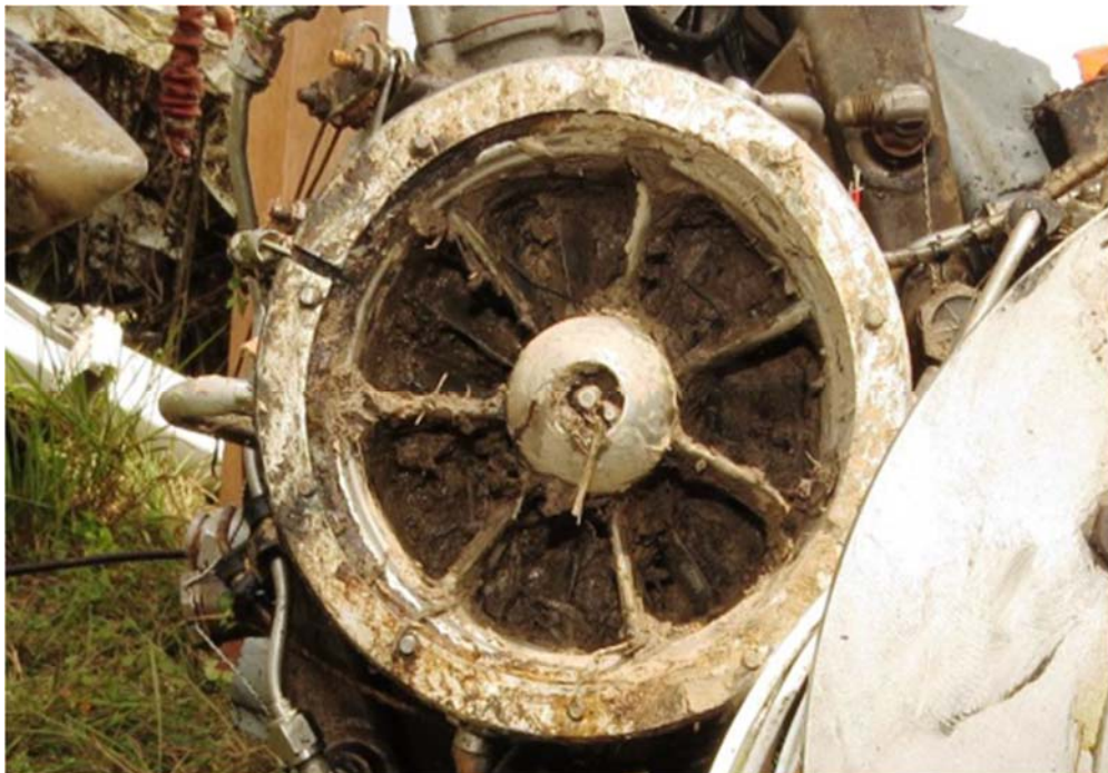
Figure 28: Right engine compressor mud extruding from compressor bleed valve
