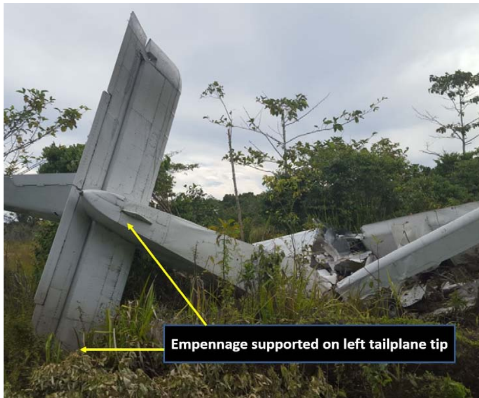
Figure 11: Empennage supported on the left tailplane tip
