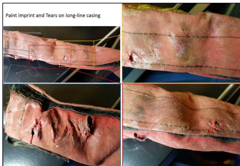
Figure 9: Sling line casing
